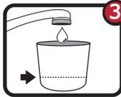
Fill Lint Trap Bucket with one inch of water and lock bucket cover onto bucket.
