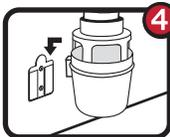
Attach Mounting Bracket on wall and slip Lint Trap Hanger into Mounting Bracket channel.
