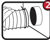
Place opposite end of LamaFlex Duct on dryer outlet and secure with provide Tension Clamp.
