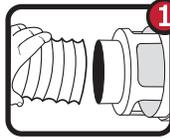
Slip LamaFlex Duct on Lint Trap Bucket Cover and secure with provided Tension Clamp about 1/4" from end.
