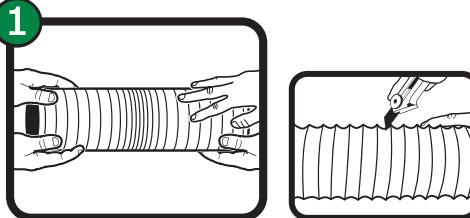
Extend duct to its full length, and position cut and discard any excess.
