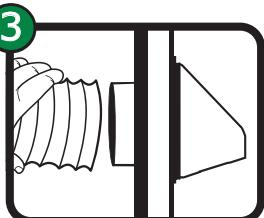
Attach the other end of flexible duct to vent pipe using supplied clamp and tighten.
