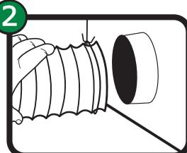
Attach one end of flexible duct to exhaust outlet pipe using supplied clamp and tighten.
