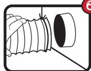
Attach one end of flexible duct to exhaust outlet pipe using supplied clamp and tighten.
