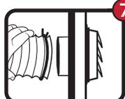
Attach the other end of flexible duct to vent pipe using supplied clamp and tighten.
