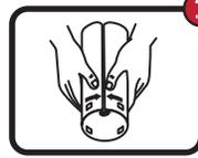
Press aluminum pipe together and lock into place.
