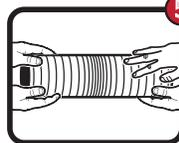
Extend duct to its full length, and position, cut and discard any excess.
