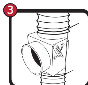
Slide flexible duct over the top and bottom openings on the Heat Economizer and secure using supplied clamps.
