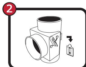
Attach mounting bracket to wall where duct was cut using 2 screws (Not Supplied). Slip Heat Economizer hanger into mounting bracket channel.
