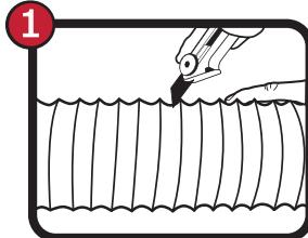
On the straightest section of flexible duct away from dryer, mark where duct will be cut. Proceed & cut duct where marked.
