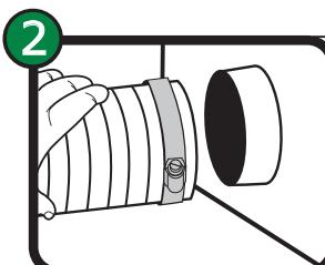
Attach one end of flexible aluminum duct to exhaust outlet pipe using supplied clamp and tighten.
