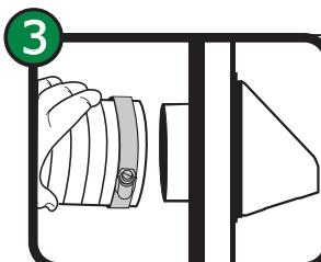
Attach the other end of flexible aluminum duct to vent pipe using supplied clamp and tighten.
