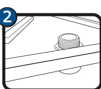
Install PVC fitting on washer tray by placing rubber washer on threaded fitting, insert through previously cut hole from bottom of tray and tighten nut. Install the assembly with PVC fitting onto the drain pipe. Position appliance in the center of the washer tray.
