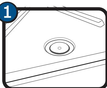
Position the washer tray to locate the embossed circle associated with the drain fitting that is closest to the appliance drain connection over the drain pipe. At the embossed circle cut a 1 ¼" diameter hole, centered within the embossment. Threaded side of PVC fitting should be a snug fit.
