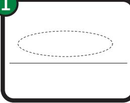
Cut a 6" hole through the outside soffit panel or use existing hole.
