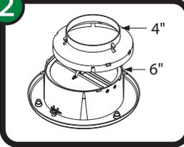
The Soffit Exhaust Vent comes assembled for use with 4" flexible duct. For use with 6" duct, simply remove and discard the 4" adaptor collar.
