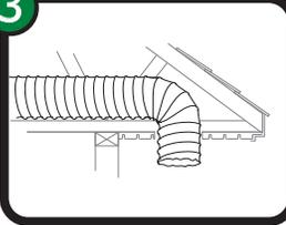
Starting from the kitchen or bathroom fan, feed the duct through the pre-cut soffit panel opening.
