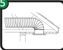
Insert the duct and Soffit Exhaust Vent into pre-cut opening making sure the facing is flush against the soffit panel.
