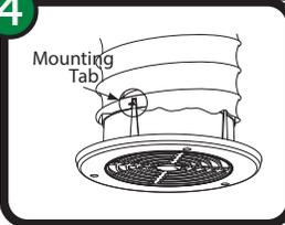
Snap the wire helix of the flexible duct over the mounting tabs on the collar of the Soffit Exhaust Vent. Seal the connection with aluminum tape.
