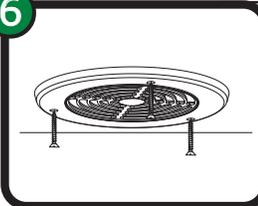
Locate, mark and pre-drill mounting holes. Fasten the Soffit Exhaust Vent to the soffit panel using the mounting screws provided.
