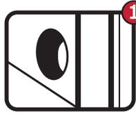
Cut a 4 1/4" hole through the outside wall or use existing hole.
