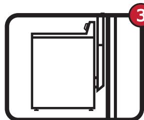
Move dryer closer to wall and slide crimped end of transition into pipe or flexible duct.
