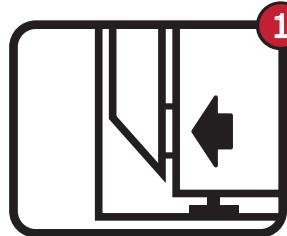
Slide non crimped end of Tite-Fit onto dryer exhaust outlet.
