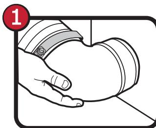
Attach existing duct to the end of the elbow using clamp provided. Using elbow with the rubber gasket side push firmly onto the clothes dryer exhaust pipe. Push dryer back until elbow makes contact with wall.
